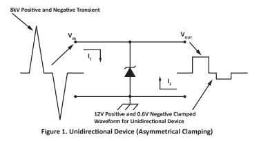
During a transient's positive cycle, the TVS diode junction is reversed biased. The diode acts in avalanche mode as the transient current  $(I_1)$  flows to ground. The transient clamps at or below the maximum clamping level provided by the TVS diode.
