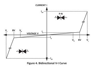
The avalanche breakdown ( $V_{(BR)}$  -  $I_R$ ) depicted on a Bidirectional V-I curve is shown in Figure 4. This is the level in which a diode will start conducting in either directions with the application of a transient (not to be confused with the maximum clamping voltage).
