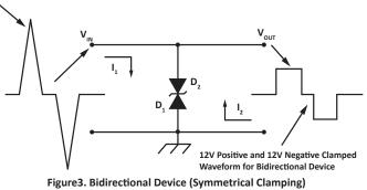
During a transient's negative cycle, D2 is reversed biased, while the other diode D1 is now forward biased. D2 acts in avalanche mode as the transient current ( $I_2$ ) is clamped at one diode drop (~12V) as the TVS conducts the transient current in the forward direction.
