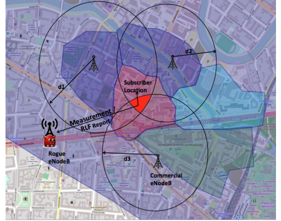
Fig. 7. Determining subscriber's precise location using trilateration (L3)
